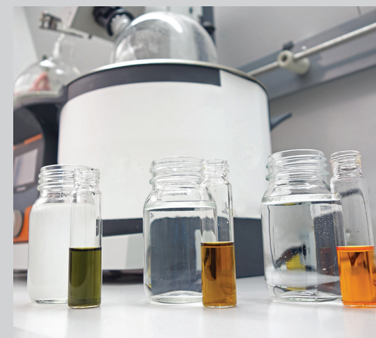
The optical COD comparison of distillate samples in the laboratory: green stands for a lot of COD, orange for little. The lighter the orange colour, the less COD is in the distillate. On the left the process water before treatment, in the middle the distillate treated with Clearcat, on the right additionally with Purecat.
