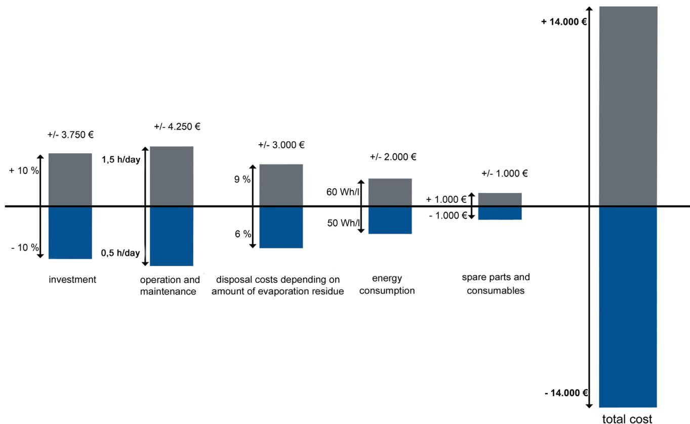
Fig. 1: Variation of operation cost of vacuum distillation systems.
